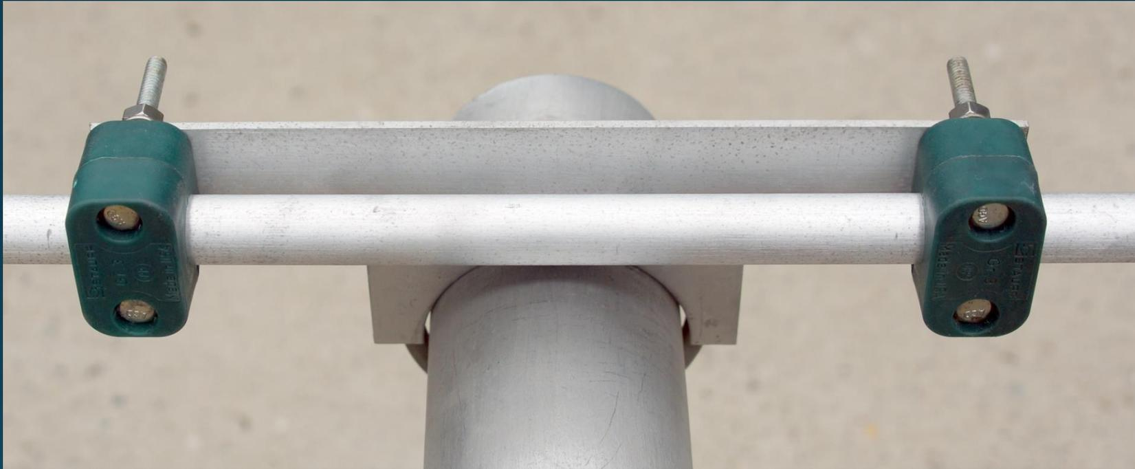
**Capacitive coupling to angle aluminum and boom are minimal, and Stauff insulating clamps are invisible to RF.**
