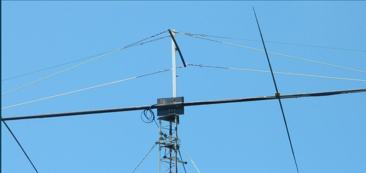
**Upper double boom truss provides both vertical and horizontal stabilization.**
