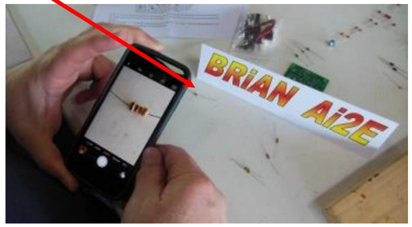
Install Resistors and leave room for a nice round bend in the leads. (No sharp bends). Use Cell Phone Application to help with color coded values of Resistors. (33K ohms)
