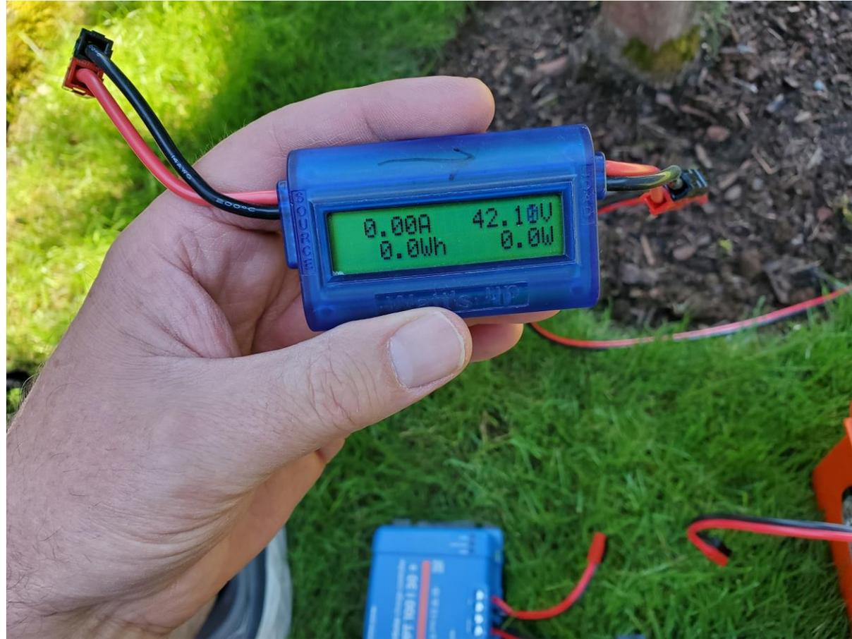
SCREEN SHOT OF "VICTRON SMARTSOLAR" CC WITH TWO 100 WATT SOLAR PANELS CONNECTED IN **SERIES**...NOTE SOLAR SIDE AND BATTERY SIDE VALUES...SOLAR INPUT VOLTAGE WENT FROM 42.1v TO 33.43v BATTERY CHARGING HAS BEGUN
