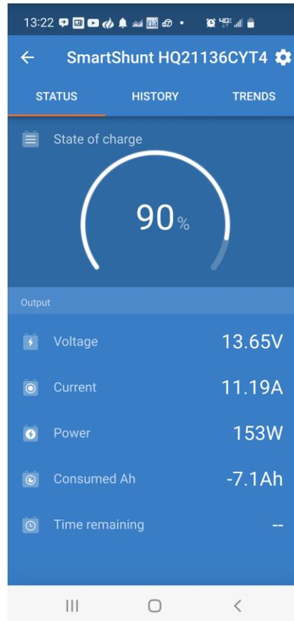
EXAMPLE OF A SCREEN SHOT OF THE “VICTRON SMARTSHUNT” ...NO SOLAR INPUT THIS TIME... JUST SHOWING A CONSTANT LOAD USING A 400 WATT INVERTER RUNNING A BOX FAN
