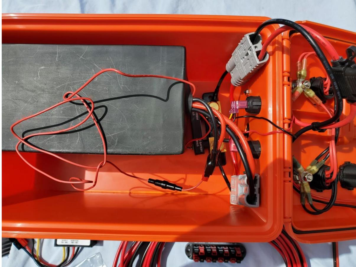
THE SMALL VICTRON SHUNT RED WIRE GIVES POWER TO THE SHUNT FOR BT USE...CONNECT THE WIRE TO THE OTHER POWER CABLE COMING FROM YOUR LFP BATTERY
