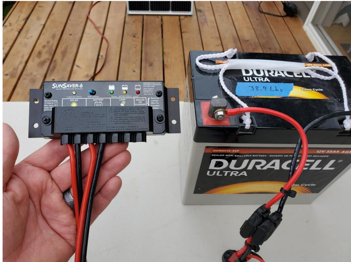
NATURE POWER 1<sup>st</sup> GENERATION SOLAR CHARGE CONTROLLER...CUT-OUT VOLTAGE IS 14.2v AND CUT-IN VOLTAGE IS 13v...8 AMP CONTROLLER...WILL “PROTECT” YOUR BATTERY
