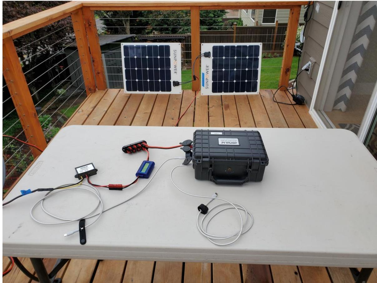
DOUBLE YOUR JOY AND CONNECT TWO MITY GO-BOXES TOGETHER...OK IF BOTH FULLY CHARGED AND SAME SIZE BATTERY IN BOTH, USING A DIYSOLAR4U SOL 20 AMP MPPT CC...MORE RF QUIET
