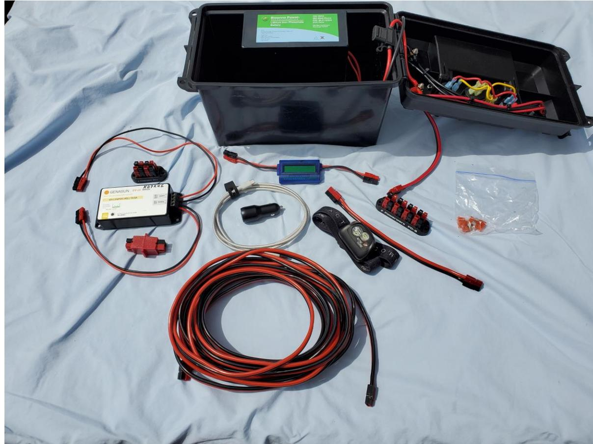
“PWRBOX” WITH SHORT CONNECTOR FROM BINDING POST TO PD-8, GENASUN GV-10, IN LINE METER, CONNECTED TO BIOENNO POWER 120 WATT “ALL WEATHER” FOLDABLE SOLAR PANEL
