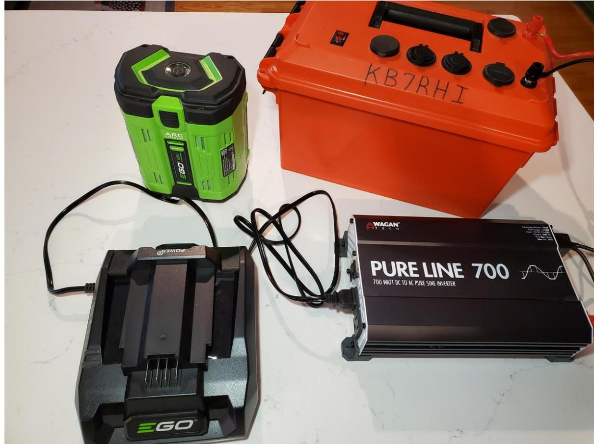
“EGO” SYSTEM 210 WATT AC CHARGER AND 700 WATT INVERTER READY TO BE HOOKED UP TO YOUR 56v LFP BATTERY
