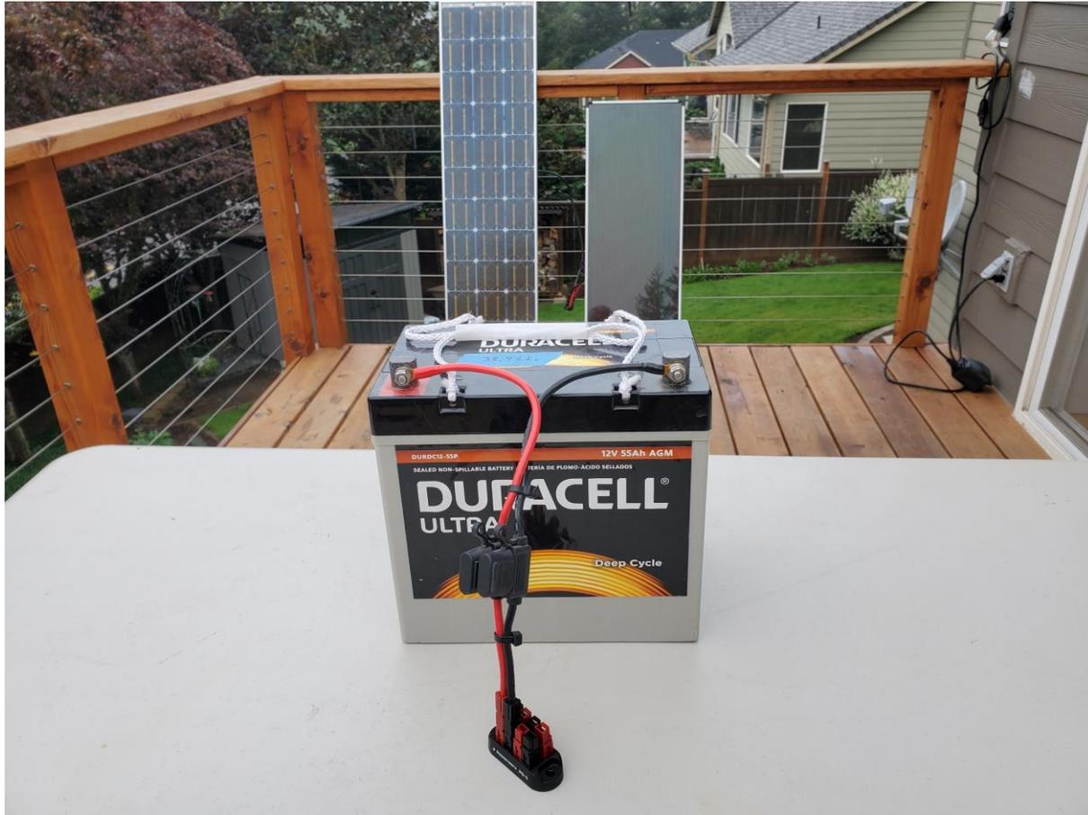
CONNECT THE CHARGE CONTROLLER TO THE BATTERY FIRST, IN LINE METER BETWEEN THE CC AND YOUR BATTERY WILL SHOW TOTAL SOLAR INPUT
