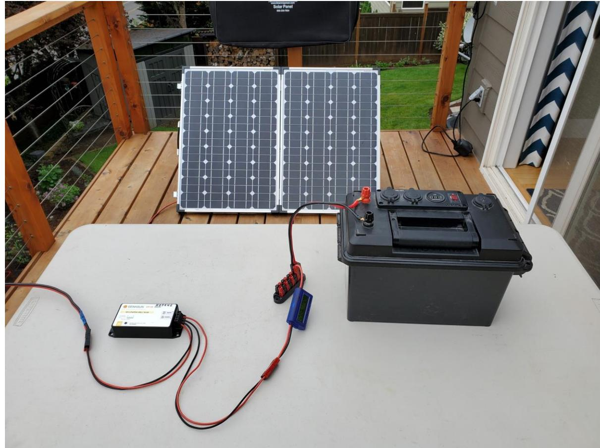
“PWRBOX” CONNECTED TO BIOENNO POWER 120 WATT FOLDABLE SOLAR PANEL WITH A POWERWERX MPPT-150 CC, GREAT FOR VHF/UHF
