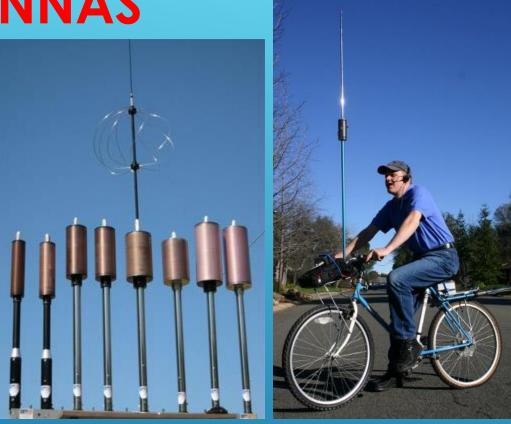
The antennas on the left are called "screwdrivers" and use a motor and wiper inside the coil to adjust the amount of loading based on frequency. The center antenna has the whip attached with a "capacitance hat" to provide capacitance to counteract inductance in the load coil and improve performance.
