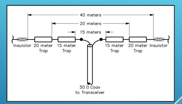
In the dipole shown, any energy on the 15m band will stop at the 15m trap and the antenna will only appear to be the width of a 15m antenna. Similarly, 20m signals will stop at the 20m traps and only see the antenna hetween the traps. Only 40m signals will pass along the entire length.
